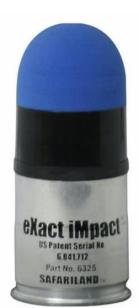
Manufacturer Description: The eXact iMpact<sup>™</sup> 40mm Sponge Round is a point-of-aim, point-of-impact direct-fire round. This lightweight, high-speed projectile consisting of a plastic body and sponge nose that is spin-stabilized via the incorporated rifling collar and the 40mm launchers rifled barrel. The round utilizes smokeless powder as the propellant and, therefore, has velocities that are extremely consistent. Used for crowd control, patrol, and tactical applications.
